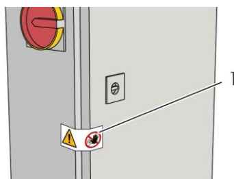
Fig. 66: Seal on switch cabinet
