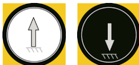
Fig. 86: Push-button for ascent and descent
