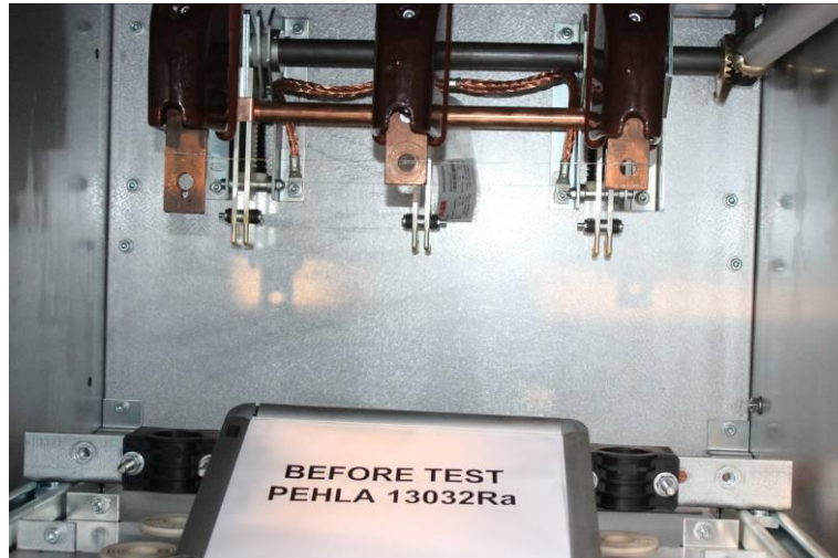
Photo No. 01 Before test PEHLA 13032Ra / 03 Initiation wire across cable terminals
