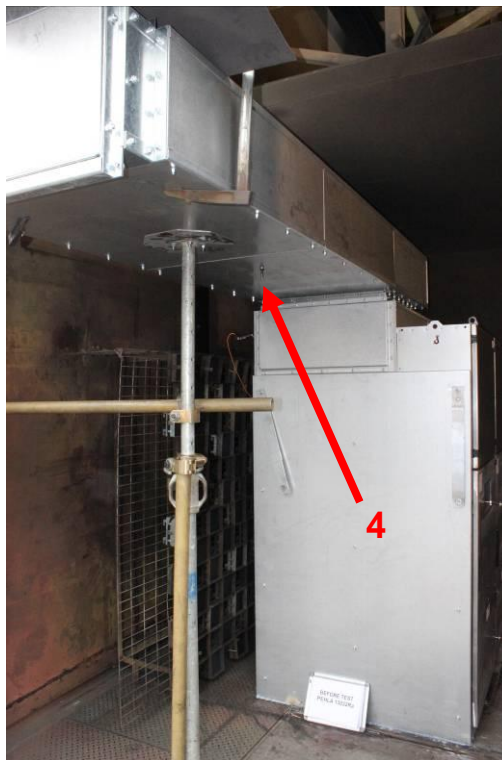
Photo No. 06 Before test PEHLA 13032Ra / 03 Test object, side view with pressure sensor 4
