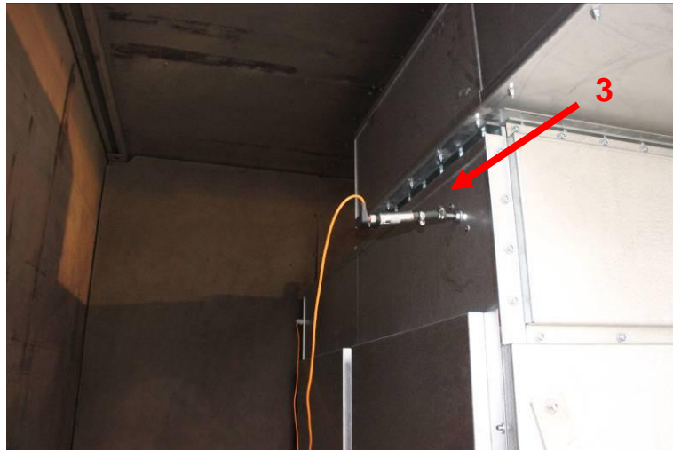
Photo No. 05 Before test PEHLA 13032Ra / 03 Test object, rear view with pressure sensor 3
