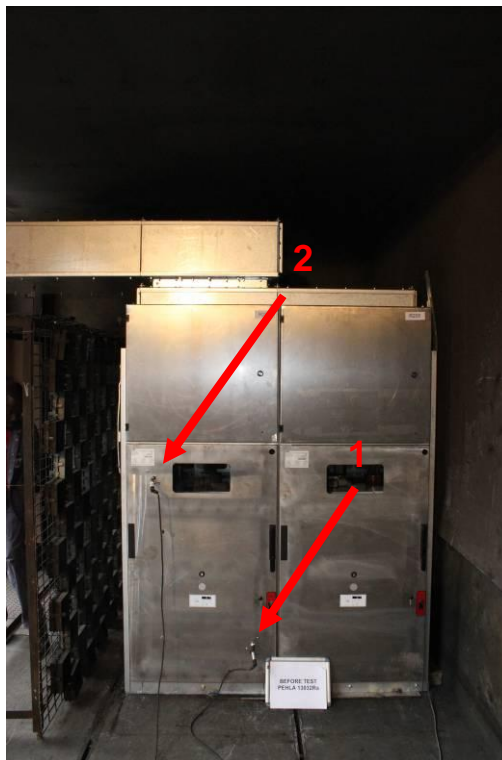
Photo No. 04 Before test PEHLA 13032Ra / 03 Test object, front view with pressure sensors 1 and 2
