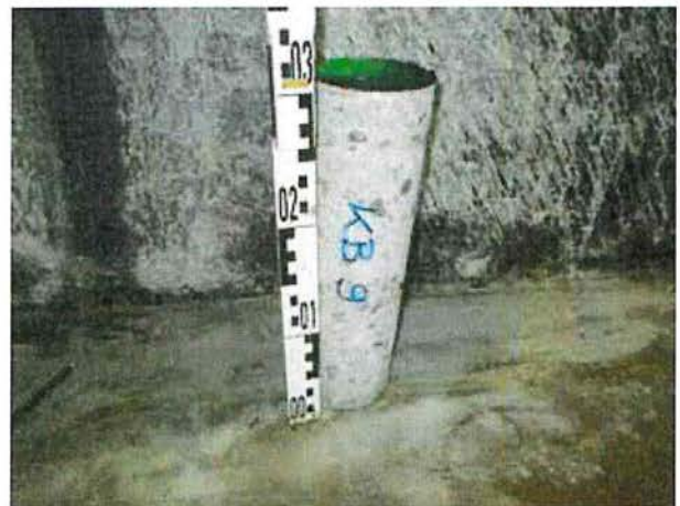
Betonbohrkern KB 9 WP
