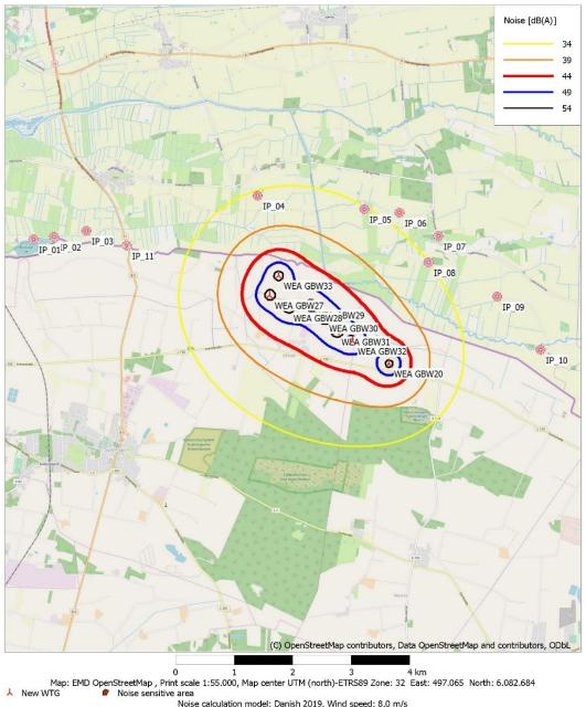
Noise calculation model: Danish 2019. Wind speed: 8,0 m/s Height above sea level from active line object
