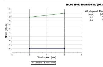
Sound level Wind speed Demands WTG noise Demands fulfilled ? [dB(A)] 42,0 [m/s] 6,0 [dB(A)]8,0 44,0 Yes
