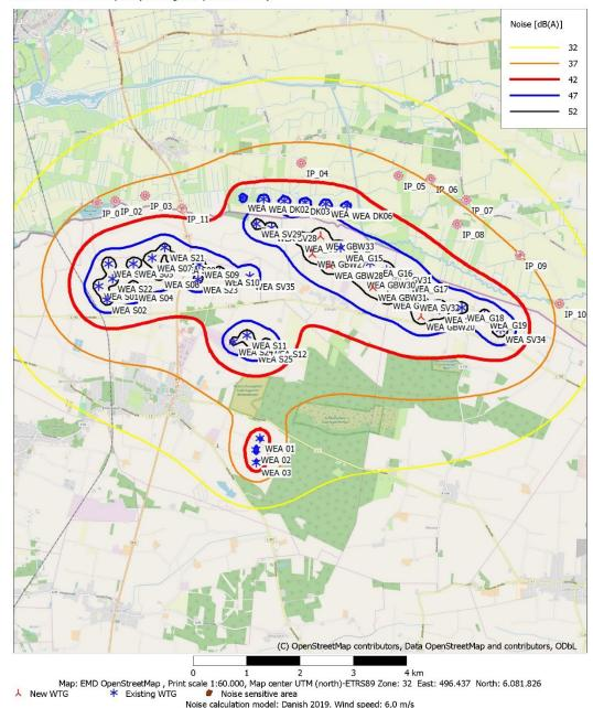
Noise calculation model: Danish 2019. Wind speed: 6,0 m/s Height above sea level from active line object
