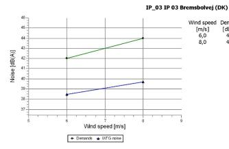
Sound level Wind speed Demands WTG noise Demands fulfilled ? [m/s] 6,0 [dB(A)] 42,0 [dB(A)] 38,4 39,7
