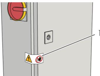
Fig. 67: Seal on switch cabinet
