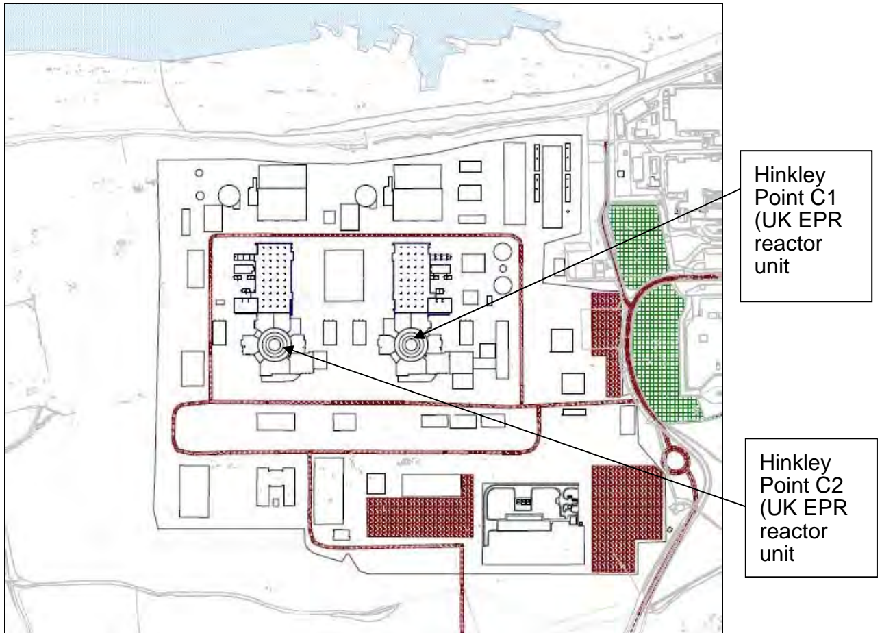
Plate 11F.4: Building model showing the layout of the proposed HPC nuclear island and ancillary buildings
