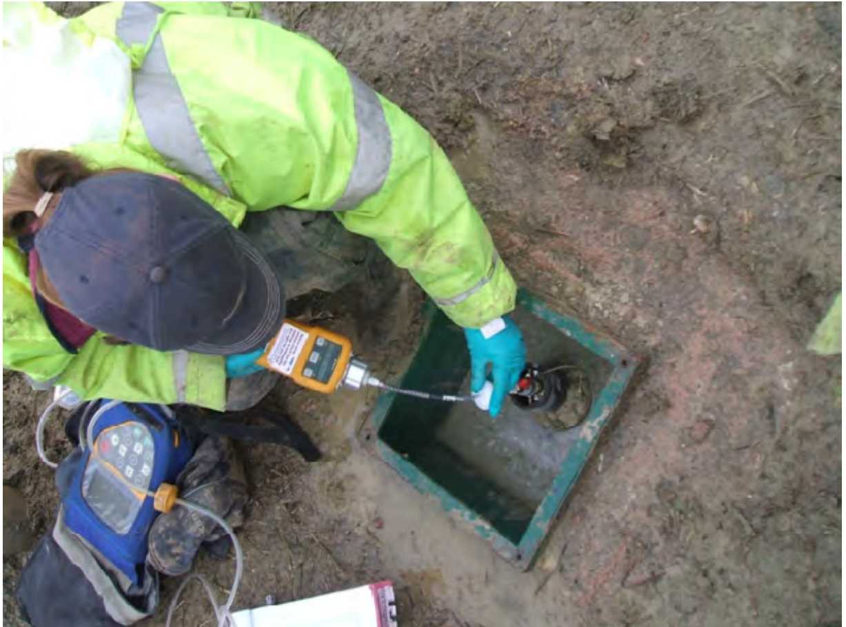
Figure 6.5: Technical Staff Undertaking Ground Gas Monitoring
