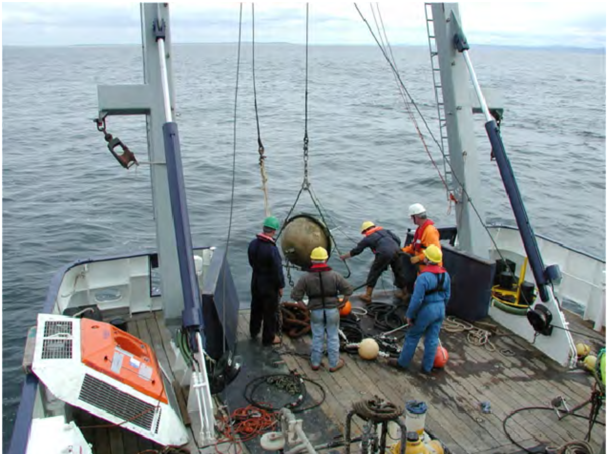
Figure 6.7: Deploying a Waverider Buoy off Hinkley Point for Data Collection
