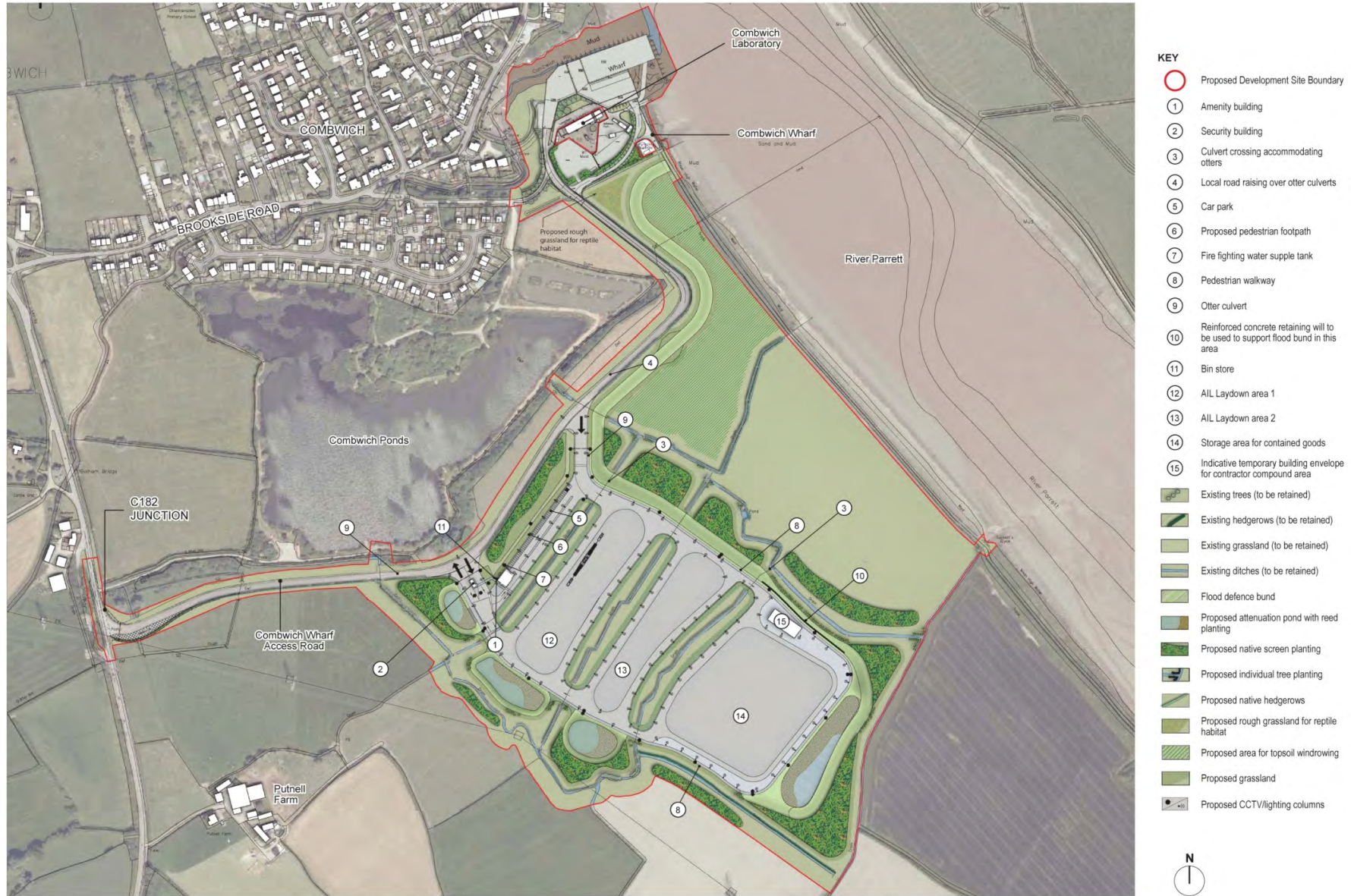
Figure 7.5: Combwich Wharf Refurbishment and Extension and Freight Laydown Facility
