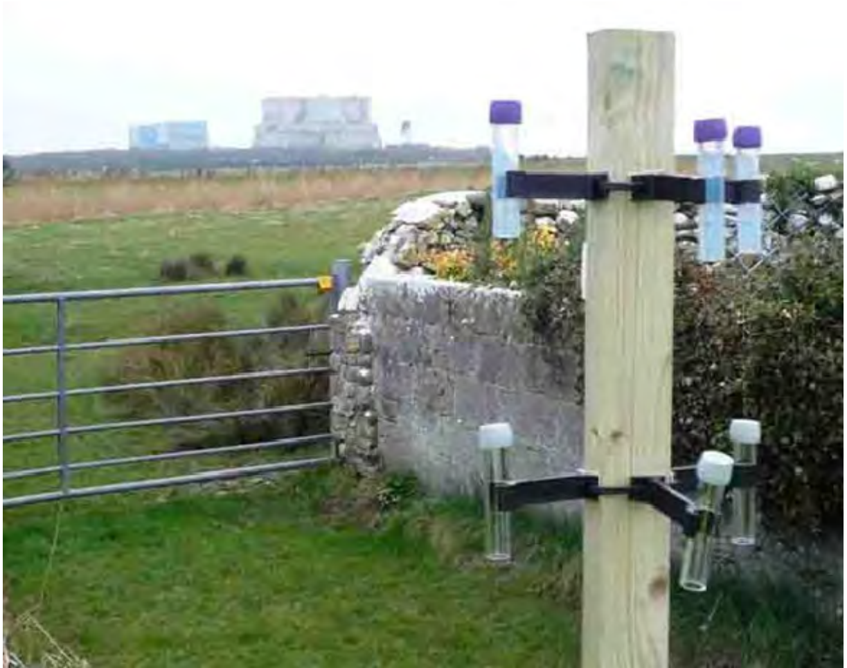
Figure 6.4: Monitoring Equipment (Diffusion Tubes) at Hinkley Point
