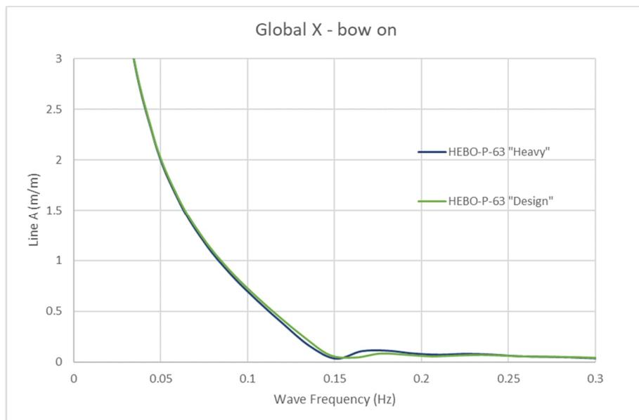
Figure 6: Comparison of surge motion RAO – Head-on waves
