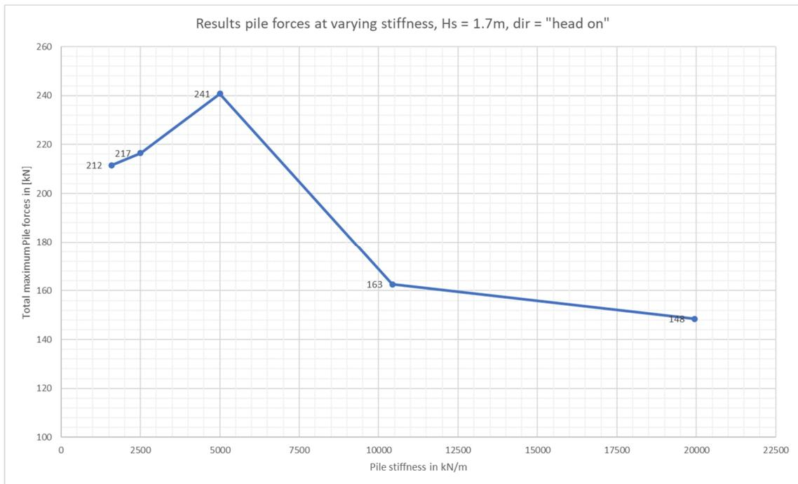
Figure 15: Total maximum pile forces at varying pile stiffness (1/10 year wave condition; head on)
