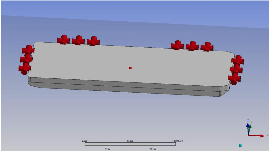
Figure 13: Model of moored pontoon with a maximum of 3 mooring piles at each side of the pontoon
