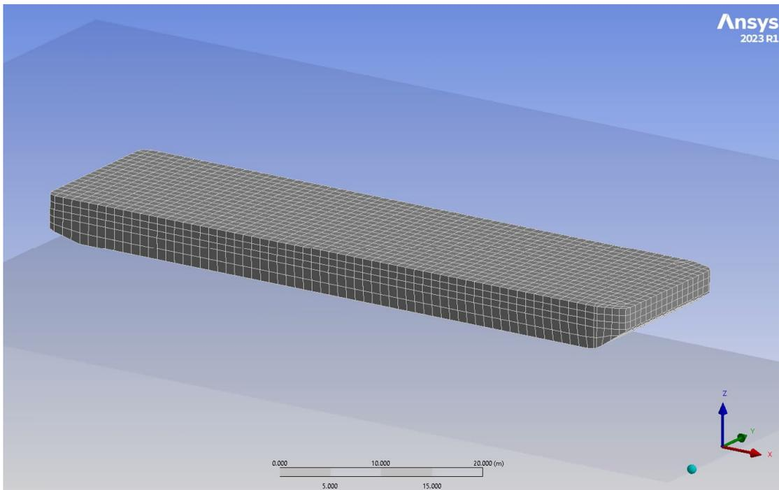
*Figure 5: Ansys AQWA model: Pontoon panel model used for hydrodynamic diffraction analysis*
