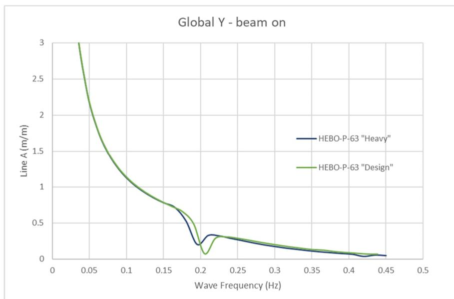
Figure 9: Comparison of sway motion RAO – Beam-on waves
