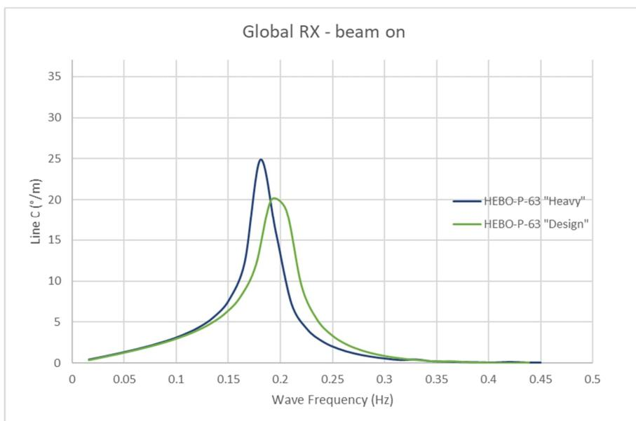
Figure 11: Comparison of roll motion RAO – Beam-on waves
