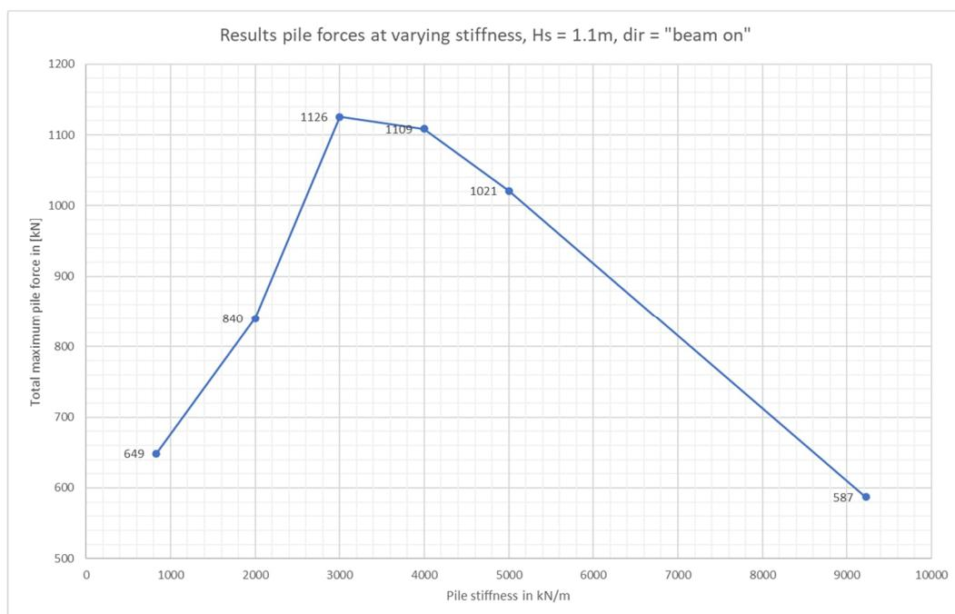
Figure 14: Total maximum pile forces at varying pile stiffness (1/100 year wave condition; beam on)
