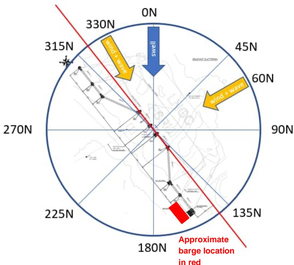
Figure 4: Barge location and main wind/wave/swell directions
