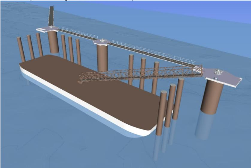
It is found that for this configuration of mooring piles and the HEBO P63 pontoon the motions of the pontoon for the stated 1:1year conditions remain within the requirements stated in section 2.
