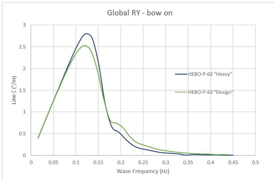
Figure 8: Comparison of pitch motion RAO – Head-on waves
