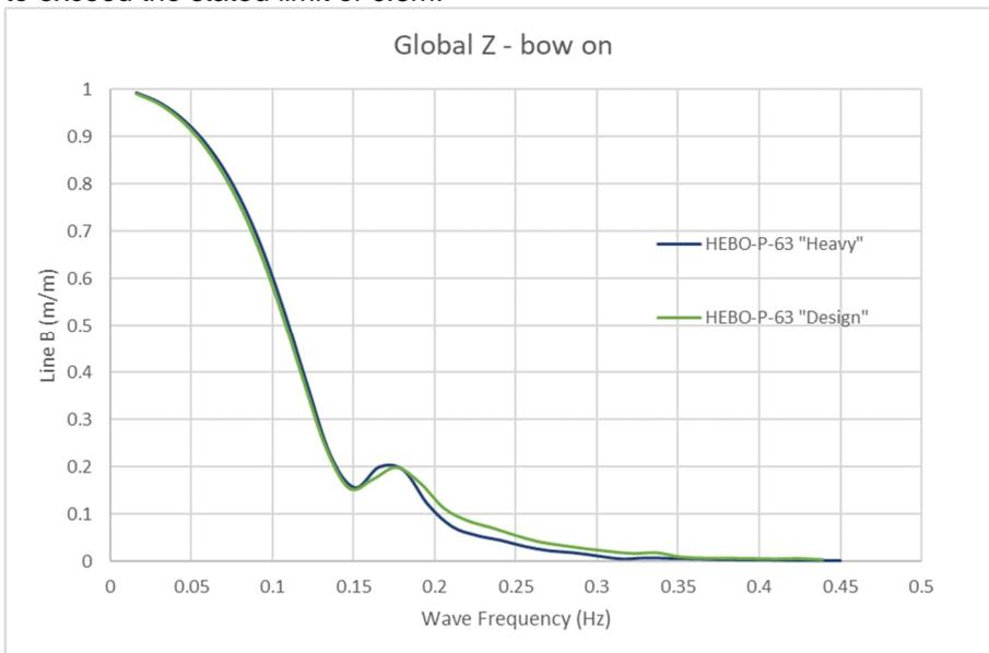
Figure 7: Comparison of heave motion RAO – Head-on waves
