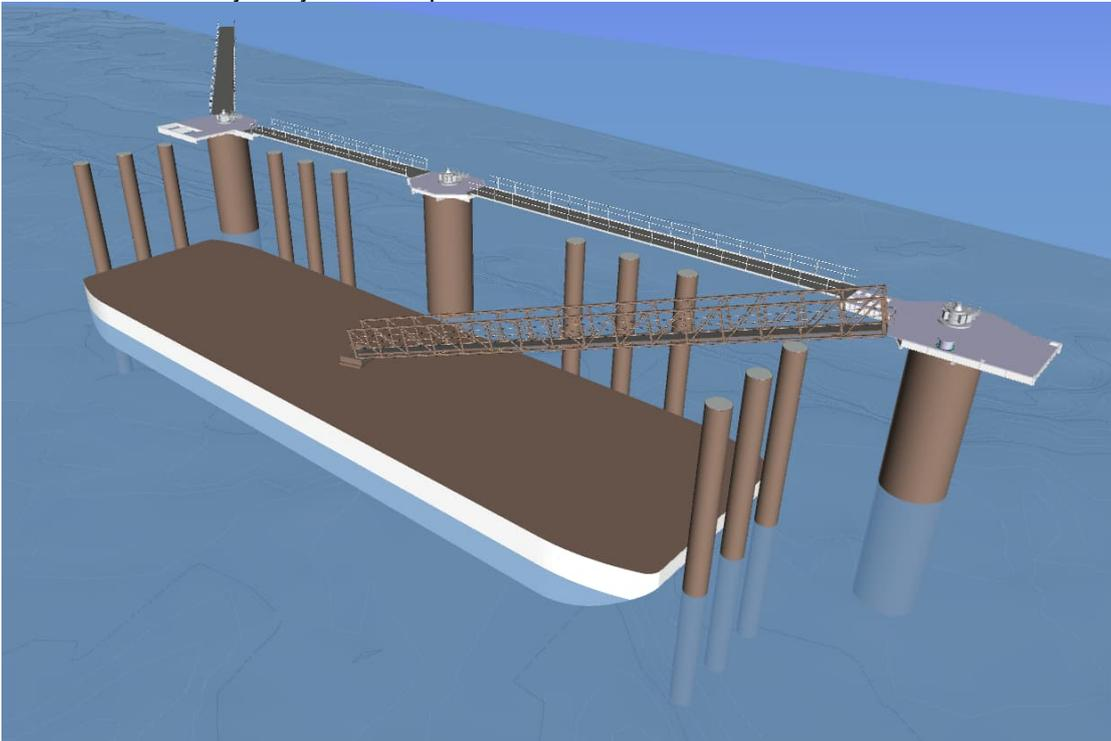
*Figure 12: Pontoon layout with piles*
