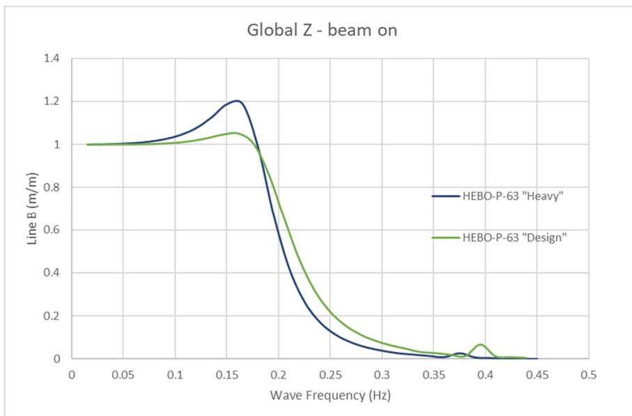
Figure 10: Comparison of heave motion RAO – Beam-on waves
