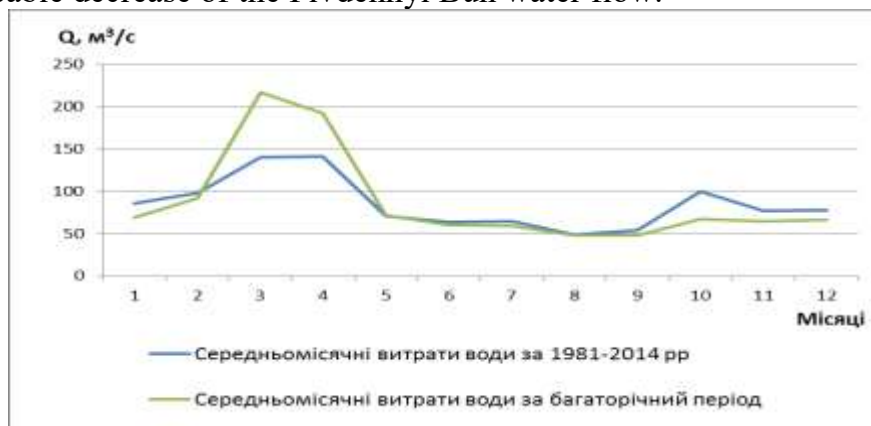
Fig. 3.14 – Graph of average monthly water flow of the Pivdennyi Buh at Olexandrivka surveillance stations
