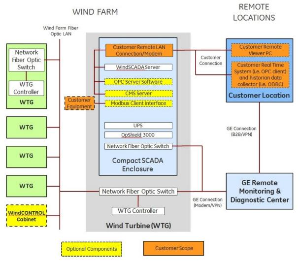
Not all components or systems may be included in a project. Drawing shows system functions, not hardware devices.
