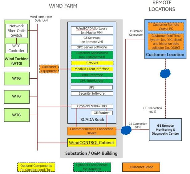
Not all components or systems may be included in a project. Drawing shows system functions, not hardware devices. \*GE Router does not apply when B2B is selected
