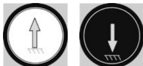
Fig. 93: Buttons for ascent and descent
