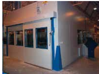
Noise enclosure, automated punching machinery, Bristol, England.
